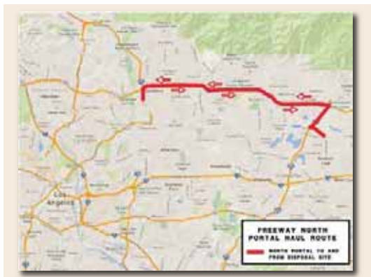
Potential haul route for the Freeway Tunnel Alternative North Portal (Single and Dual-Bore)
